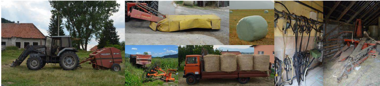
Figure 52: classic equipment on a medium family dairy farm (tractor with round baler, mower, haybale, windrower, truck with round bales, milking machine, corn silage harvester). Anouk Fraisse.
